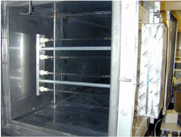
Figure 2-1. Ballast box installed on the outside of the test rig.
