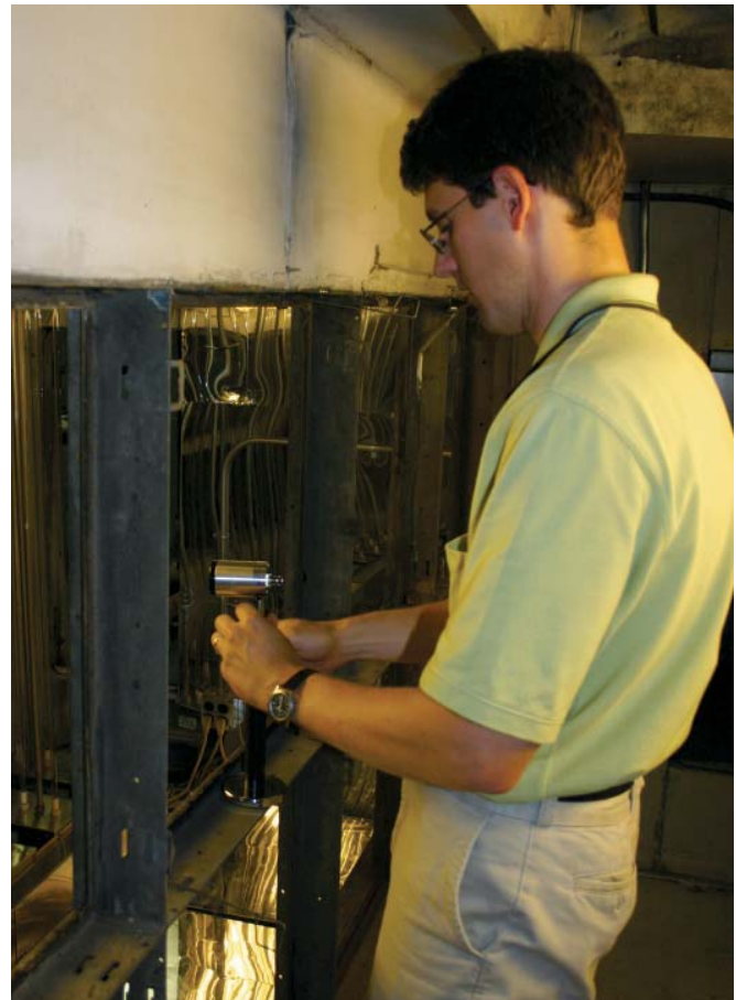
Figure 5. An LRC researcher positions a UV sensor in the plenum opening.
